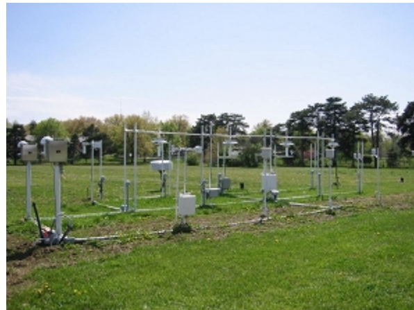
Fig. 1. Instrumentation illustration: the array of RH and dew point temperature sensors used (two HMP45C inside the USCRN shields, two HMP45C inside the Gill shields, HMP233 sensors and MP101A sensors in the USCRN shields) at the experimental field.
