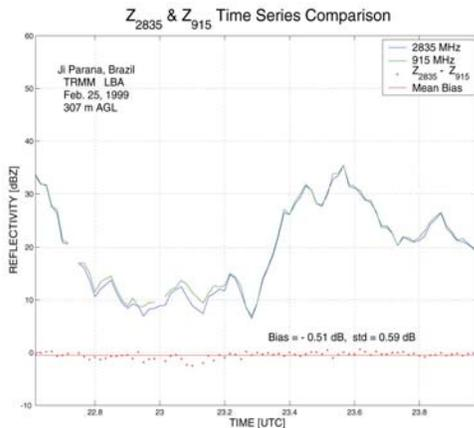
**Figure 4: Overlaid time series of  $Z_{2835}$  versus  $Z_{915}$  over an hour and a half of TRMM-LBA, demonstrating the close agreement between the two systems.**
