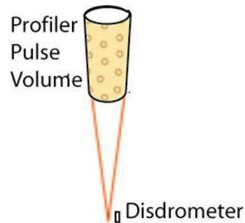
**Figure 1:** Schematic depiction of the profiler calibration set up. Gage et al. provide a picture of a typical site and typical system parameters in the companion paper 10.6. Williams et al., paper 11.3, discuss using these systems to calibrate scanning radars.
