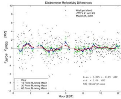
**Figure 5: Difference in Z values from two disdrometers 1 m apart.**
