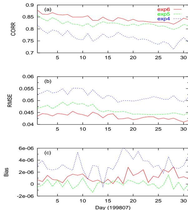
Figure 1: Statistical results of the ANN soil moisture estimation from July 1998. Variables are (a) correlation between the ANN model estimate and LDAS soil moisture, (b) Root mean square error, and (c) bias defined as the difference between the model estimate and LDAS soil moisture with line types as labeled. LDAS data is used as the "ground truth" for soil moisture in this study.
