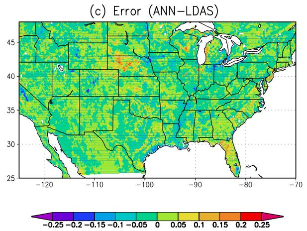
Figure 2: Statistical results of the ANN soil moisture estimation from July 1998. Variables are (a) correlation between the ANN model estimate and LDAS soil moisture, (b) Root mean square error, and (c) bias defined as the difference between the model estimate and LDAS soil moisture with line types as labeled. LDAS data is used as the "ground truth" for soil moisture in this study.
