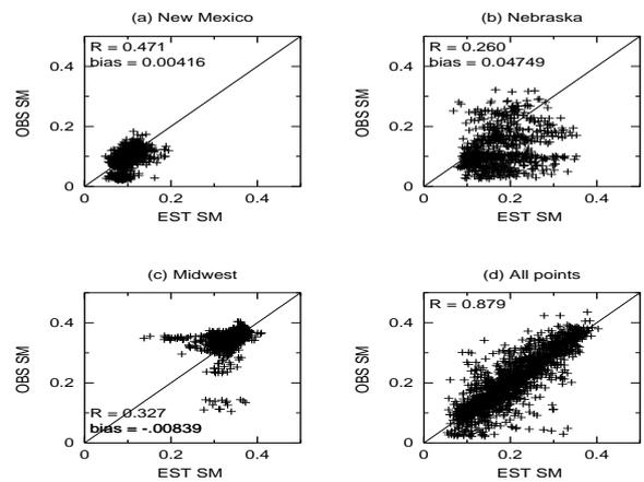
Figure 3: Scatter plots of estimated and observed soil moisture for different regions as labeled for 1 July 1998. Solid line represents points where the estimated soil moisture equals to that of observed.
