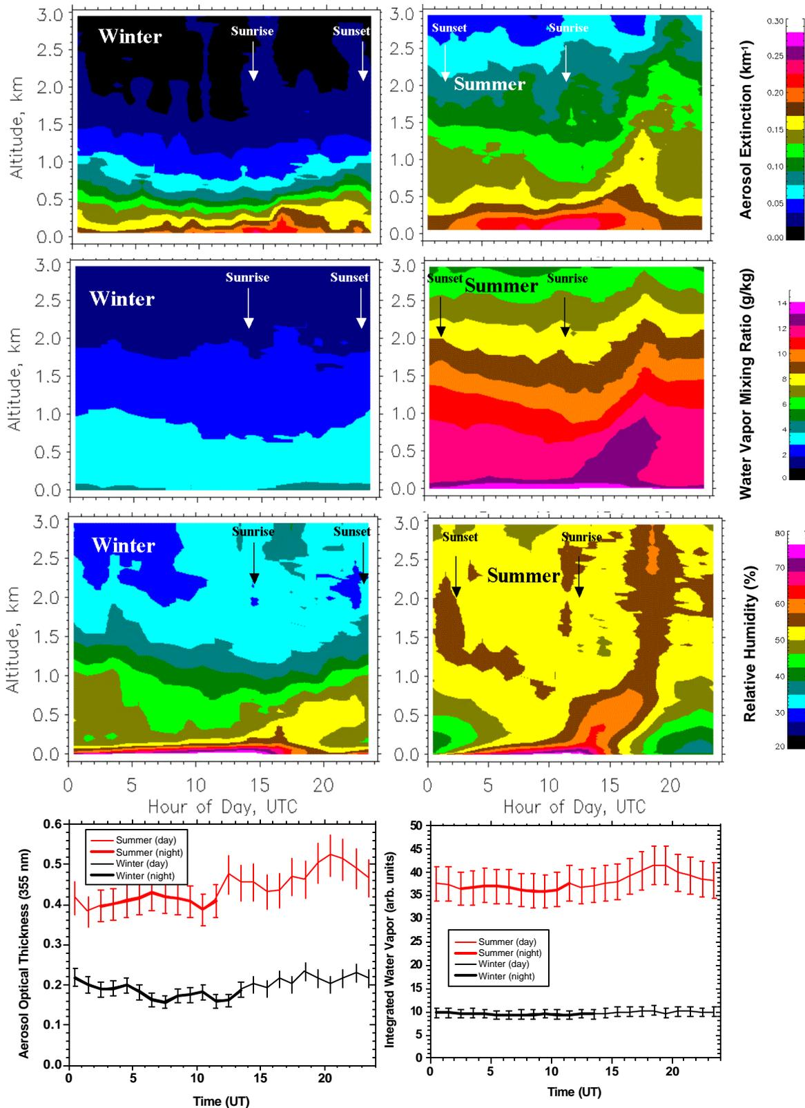
Figure 3. (top) Images showing average diurnal variation of aerosol extinction (top), water vapor mixing ratio (middle), and relative humidity (bottom) profiles measured by CARL for winter (left) and summer (right). (bottom) average AOT (left) and integrated water vapor (between 0 to 3 km) (right) for summer and winter.
