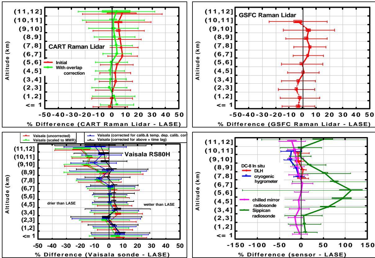
Figure 1. Average differences (%) in water vapor measurements between various AFWEX sensors and LASE. Thick rectangles (boxes) represent  $\pm 2$  st. error of the average; error bars represent standard deviations of the measurements. Note the change in scale for the comparisons on the bottom right.
