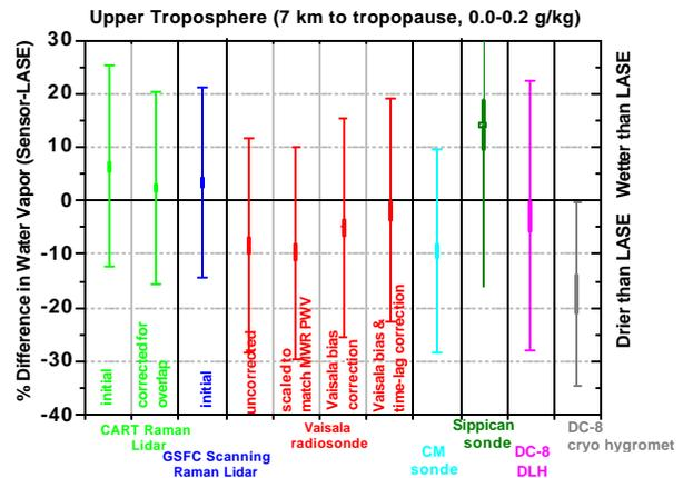
Figure 2. Average differences in UT water vapor measurements referenced to the LASE measurements. Thick black rectangles (boxes) represent +/- 2 st. deviations of the average and error bars represent standard deviations of the measurements.
