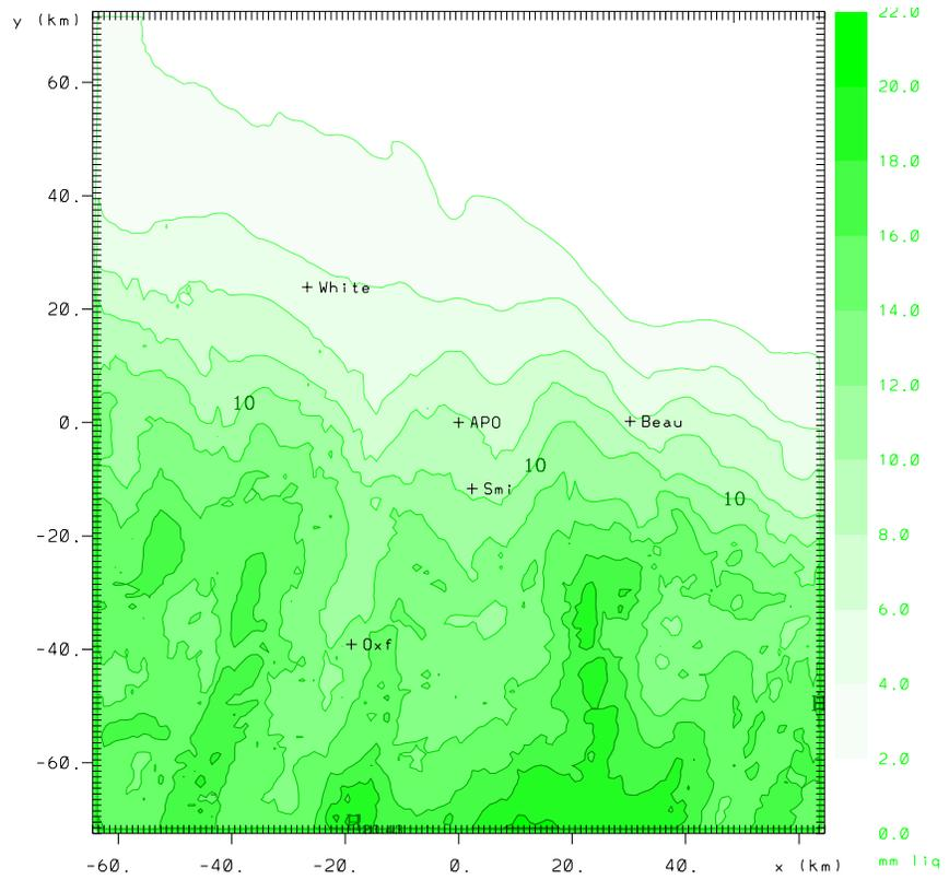
Figure 4. Total accumulated precipitation on grid 4 at 0800 UTC 3 March 2000. Vertical grid spacing is 200 m. Contour interval is 2 mm.
