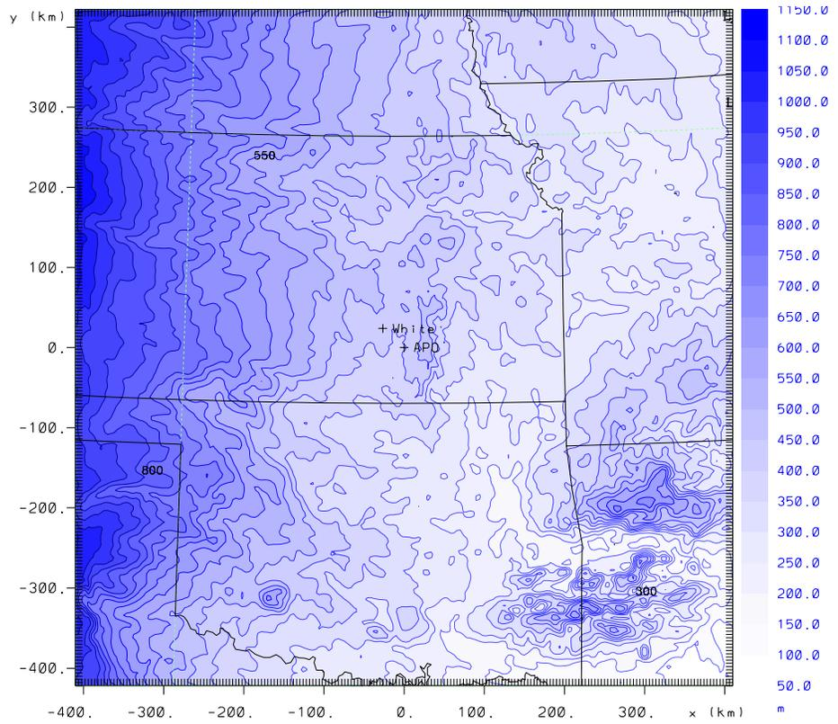
Figure 2. Topography represented on grid 4 of the RAMS simulations. Contour intervals are 20 m.
