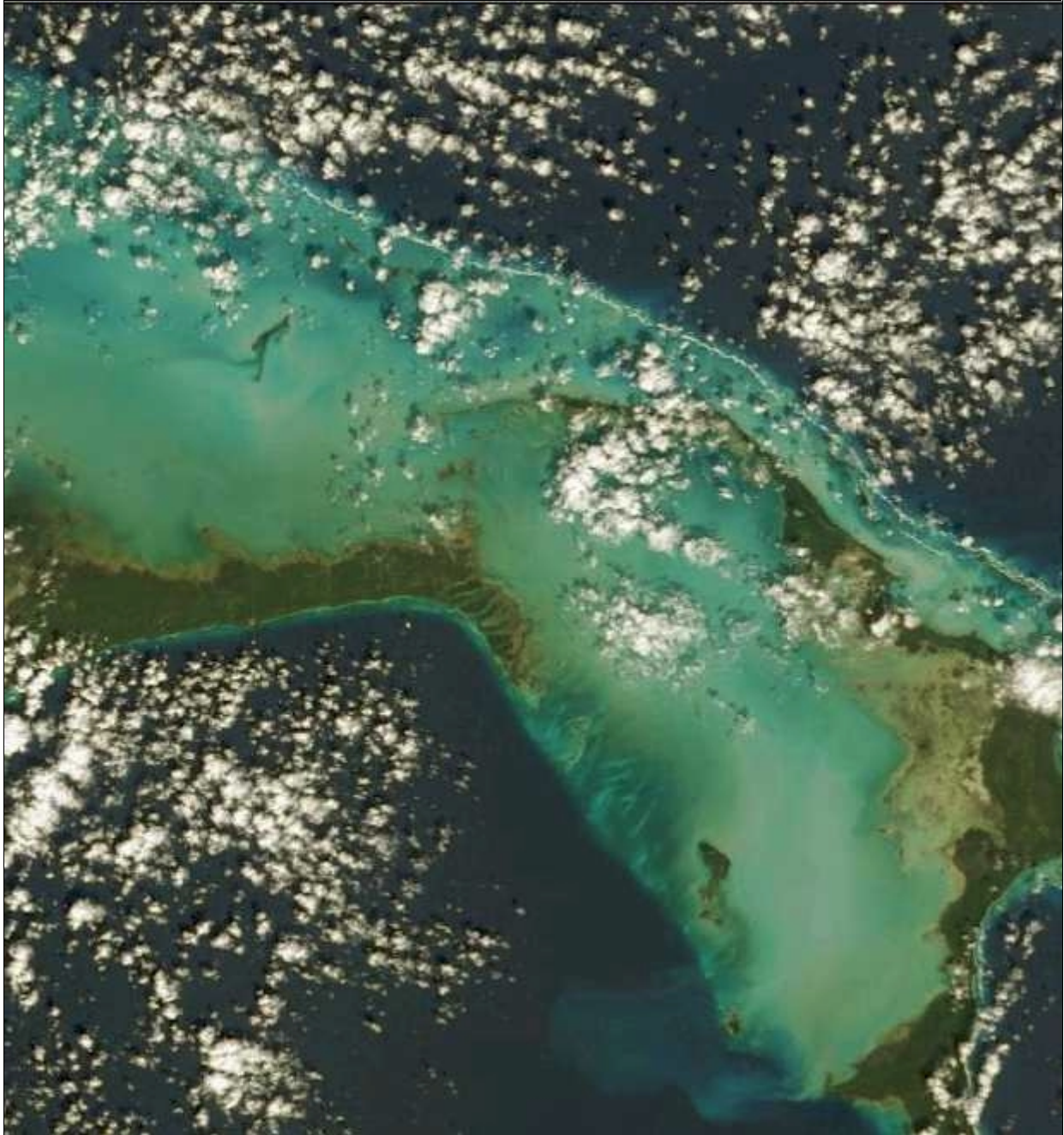
Figure 5a. MODIS Terra L1B true color image (red: band 1 (.65 \mu\text{m} ), green: band 4 (.55 \mu\text{m} ), blue: band 3 (.46 \mu\text{m} ) processed with IMAPP from data collected at the University of Wisconsin - Madison over the Bahamas on 6 November 2001.
