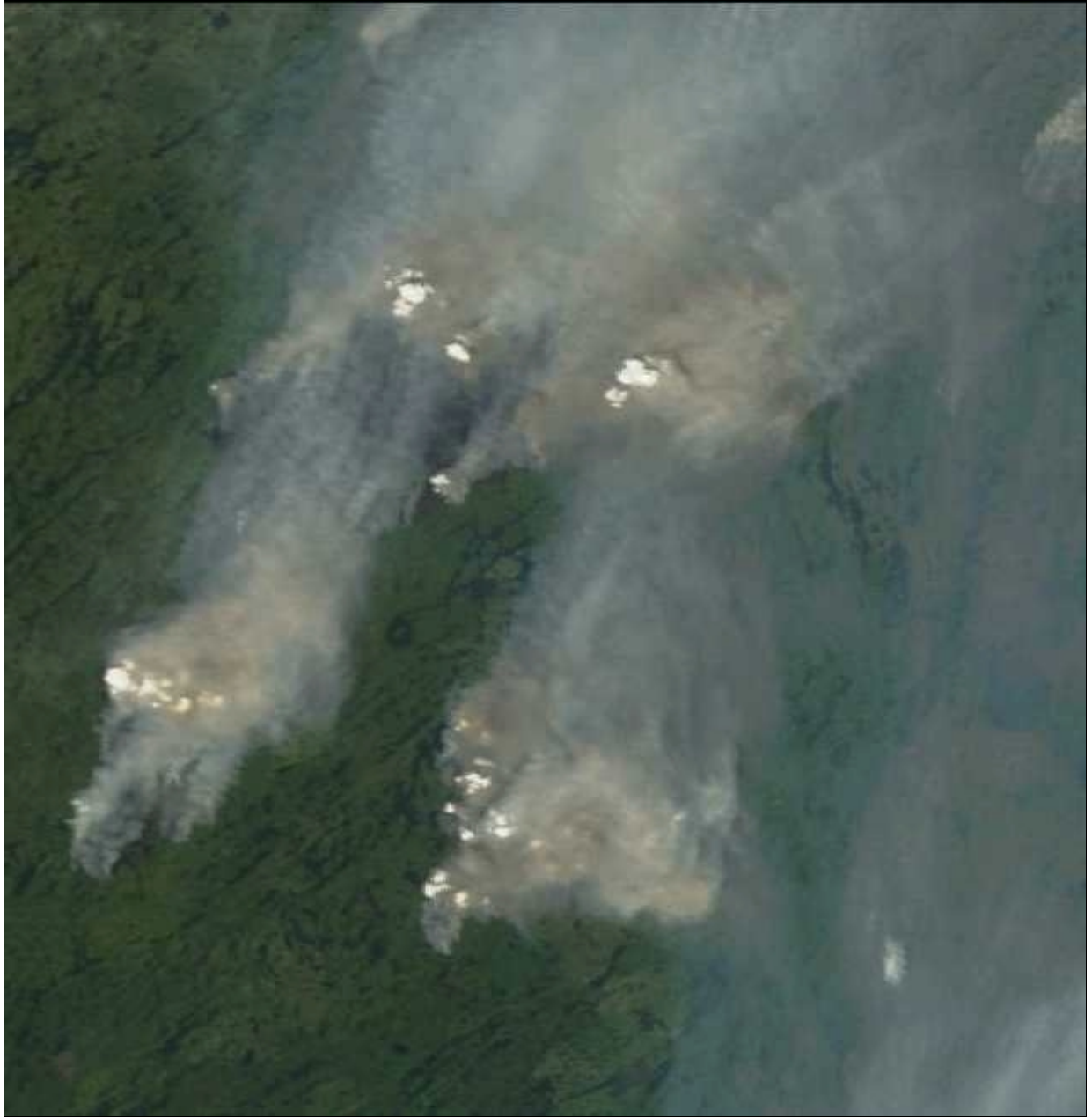
Figure 5b. MODIS Terra L1B true color image (red: band 1 (.65 \mu\text{m} ), green: band 4 (.55 \mu\text{m} ), blue: .band 3 (.46 \mu\text{m} ) processed with IMAPP from data collected at the University of Wisconsin - Madison over forest fires in Saskatchewan, Canada on 27 June 2002.
