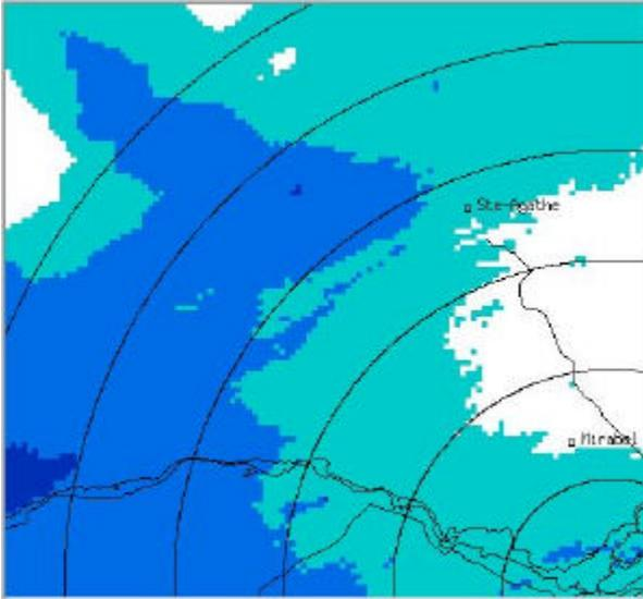
Figure 11 - Northwest portion of McGill radar coverage with C3 correction level showing a lower degree of shadowing by the two hills northwest of the radar, which is located in the lower right corner (February 1, 2002, 11:00 UTC)
