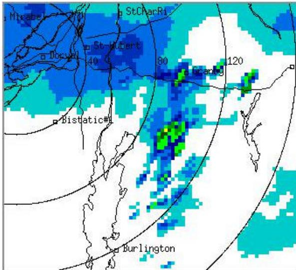
Figure 2 - Southeast portion of McGill Radar coverage showing bright spots associated with Green Mountains (radar is located in upper left corner) (February 20, 2002, 21:00 UTC)
