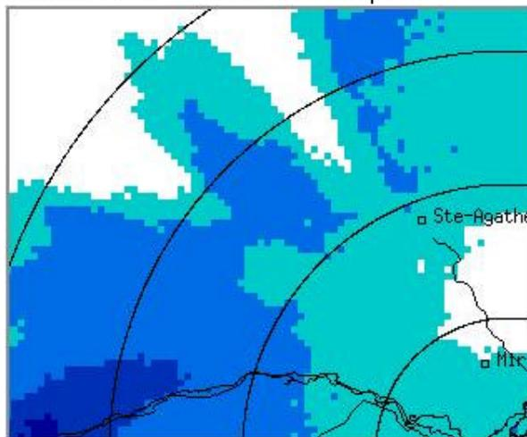
Figure 1 - Northwest portion of McGill Radar coverage showing the V-shaped shadows of the two hills northwest of the radar, which is located in the lower right corner (February 1, 2002, 11:00 UTC)
