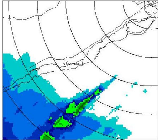
Figure 13 - Southwest portion of McGill Radar coverage with C3 correction level showing that the bright spots associated with anomalous propagation were decreased and the thin V-shaped shadow was filled in (radar is located in upper right corner) (February 21, 2002, 1:00 UTC)
