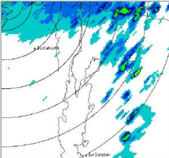
Figure 12 - Southeast portion of McGill Radar coverage with C3 correction level showing that the "bright spots" of the Green Mountains were decreased (radar is located in the upper left corner) (February 20, 2002, 21:00 UTC)
