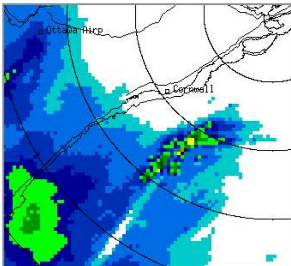
Figure 3 - Southwest portion of McGill Radar coverage showing bright spots and thin V-shaped shadow associated with anomalous propagation (radar is located in upper right corner) (February 21, 2002, 1:00 UTC)
