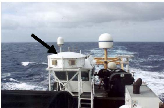
Fig. Electronically stabilized phased-array 915-MHz antenna: NOAA R/V Ronald H. Brown (arrow).
