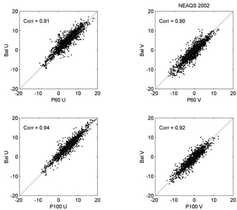
Fig. 4 U/V Horizontal wind component scatter plots NEAQS 2002. Radar wind profiler vs rawinsonde: 60 and 100 m modes, for all heights.
