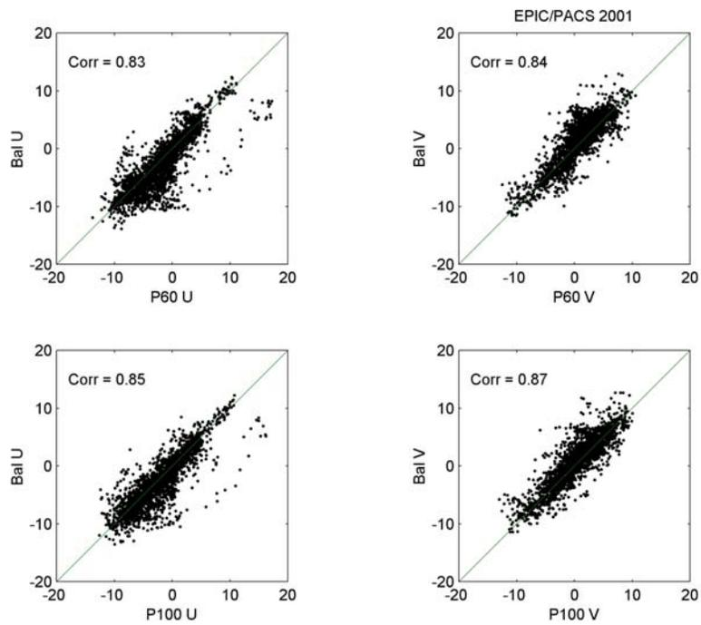
Fig. 3 U/V Horizontal wind component scatter plots EPIC/PACS 2001. Radar wind profiler vs rawinsonde: 60 and 100 m modes, for all heights.
