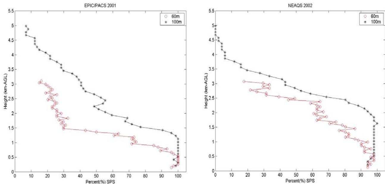
Fig. 5 Number of good radar wind profiler data pts at each height (%): left EPIC/PACS 2001, right NEAQs 2002.
