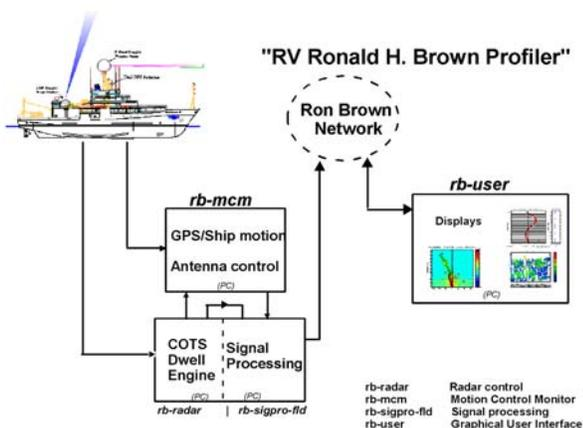
Fig 2. Schematic of the entire radar wind profiler system.
