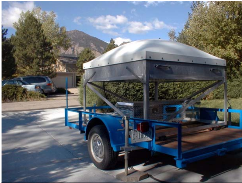
Figure 1 Photograph of the mobile wind profiler deployed in a severe clutter environment.
