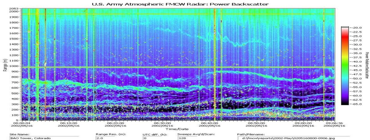
**Figure 6** Clear-air turbulence with point targets. Insects appear as dots while birds cause saturation of the receiver causing vertical streaks. (0-2053 meters, 2 hours left-to-right, May 16, 2002, Erie CO)
