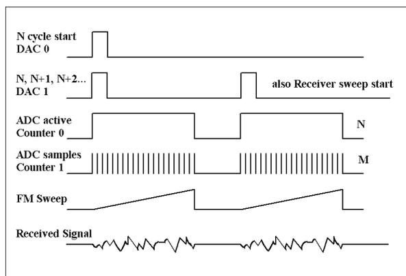
Figure 3 Basic FM-CW radar control and timing.
