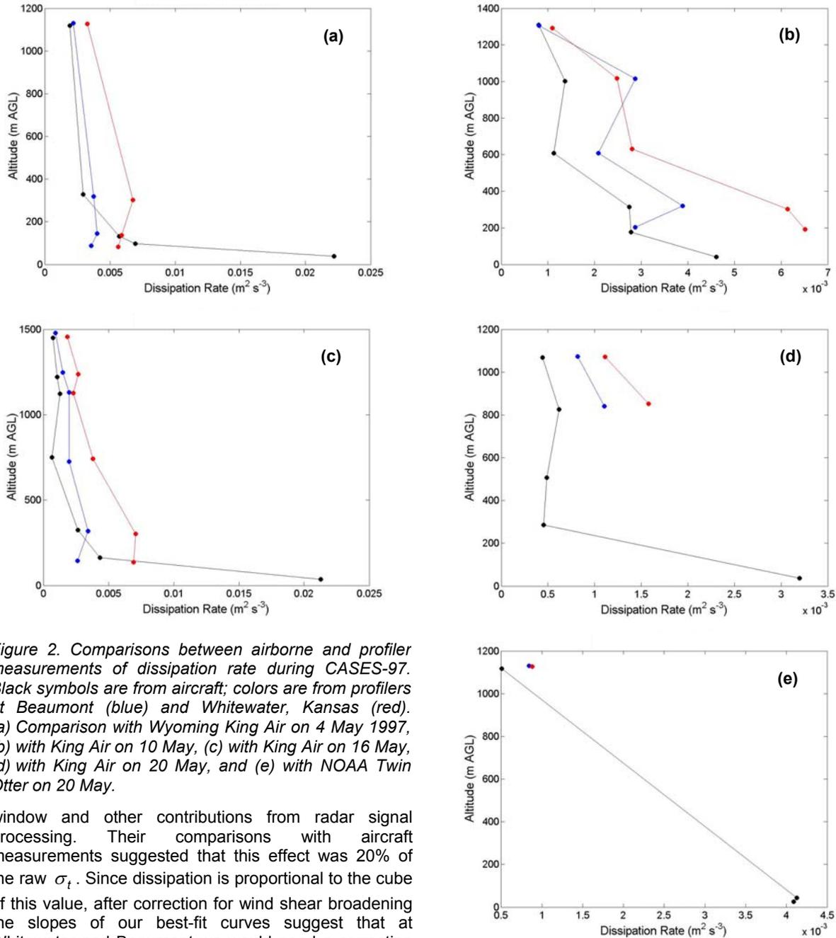
Figure 2. Comparisons between airborne and profiler measurements of dissipation rate during CASES-97. Black symbols are from aircraft; colors are from profilers at Beaumont (blue) and Whitewater, Kansas (red). (a) Comparison with Wyoming King Air on 4 May 1997, (b) with King Air on 10 May, (c) with King Air on 16 May, (d) with King Air on 20 May, and (e) with NOAA Twin Otter on 20 May.
