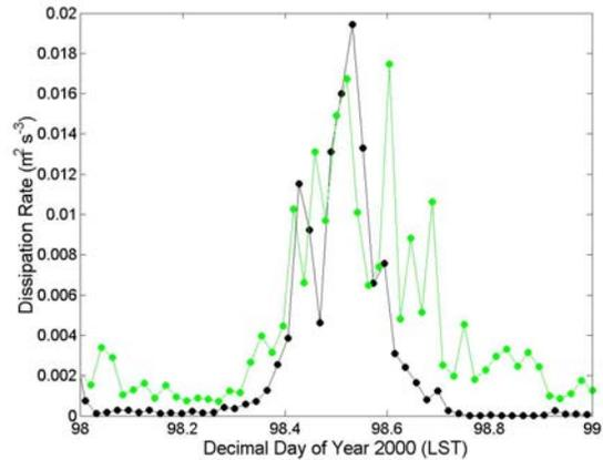
Figure 1. Time series of dissipation rate measured by a sonic anemometer (black) mounted 120 m above the surface and the lowest range gate of a wind profiling radar (green).
