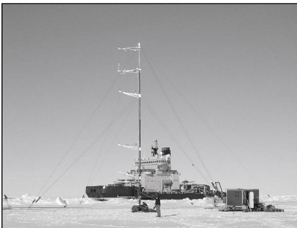
Figure 7. The 18-m telescopic mast, with profile and turbulence instrumentation. In front of the mast is the mandatory bear guard and to the right is the electronics hut. Oden is ~300 m away in the background.
