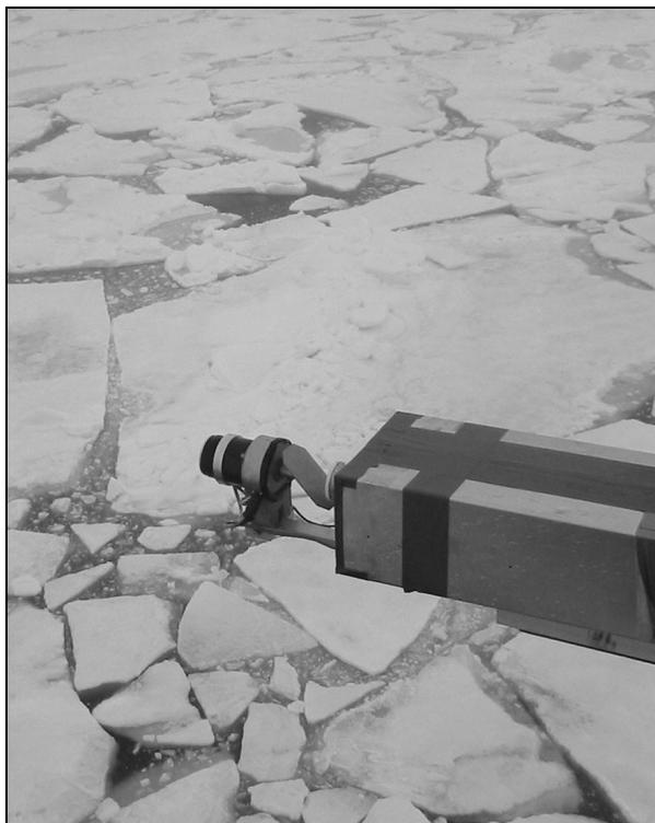
Figure 4. Scanning microwave radiometer mounted on the starboard side of the 7<sup>th</sup> deck, with a free view over the ocean.
