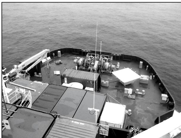
Figure 3. View of the Oden foredeck from the topmost 7<sup>th</sup> deck, showing the square-shaped antenna for the NOAA/ETL 915MHz Wind Profiler, and the round antenna for the S-band cloud radar partly hidden aft of the forward container housing the electronics for both systems.
