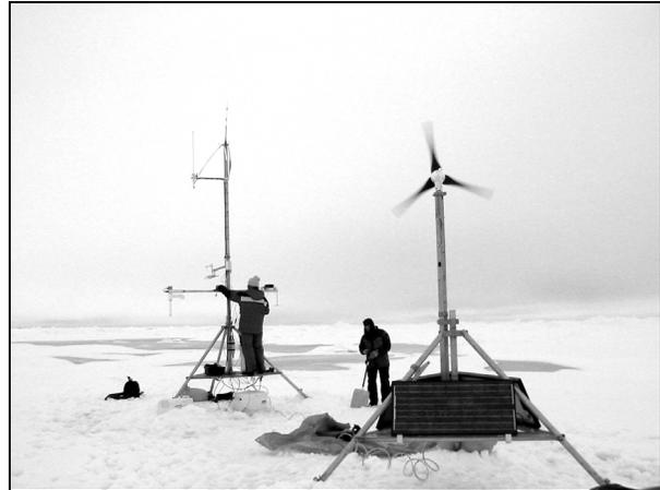
Figure 8. Deployment of a PAM-station instrument stand (background), carrying one sonic anemometer and instruments for measuring mean temperature, humidity, and atmospheric pressure. The instruments are powered by batteries, fed by solar panels and a wind generator on the separate stand in the foreground.
