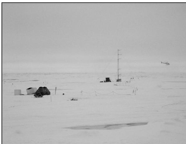
Figure 5. View of the ice-camp instruments, showing the Sodar and tethered sounding site in the foreground to the left and the tower site further back. Also seen is the helicopter that was sometimes used for aerosol profile measurements.
