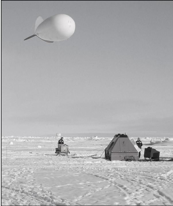
Figure 6. View of the tethered sounding system, with the kytoon being launched with the aerosol pack (visible just at the horizon).
