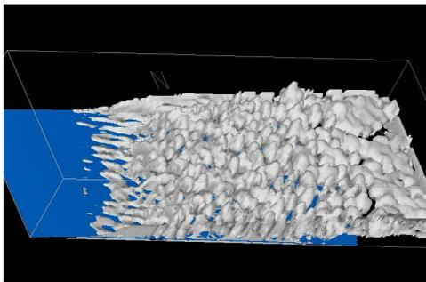
Fig. 4 Three-dimensional depiction of the model cloud outline for total water content of 0.1 g/kg from the 0.55 km model.
