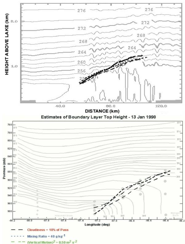
Fig. 5 Profiles of potential temperature and estimated boundary layer height across the lake a) Simulated, b) Observed (from Kristovich *et al.*, 2003). Thick gray lines at bottom indicate areas over land.
