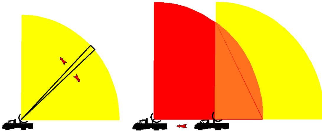
Fig. 3 – Schematic of Stationary RHI (left) and Rolling RHI (right) scanning strategy
