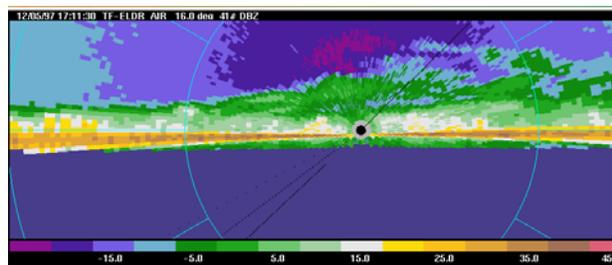
Figure 2. ELDORA observations of radar reflectivity at 1711 UTC on 5 December. These data were taken with the forward radar, at 18 deg from the vertical.
