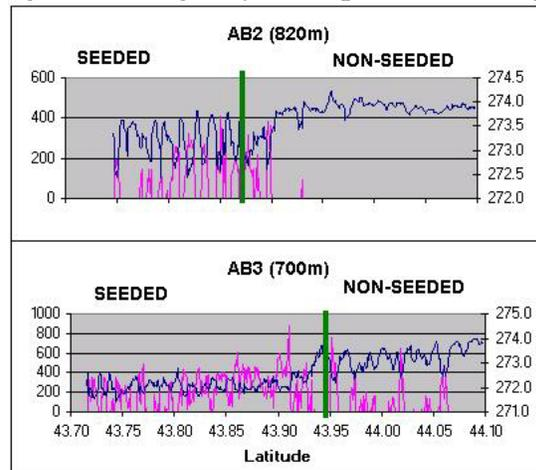
Figure 3. King Air time series of potential temperature (blue; scale at right in K) and total FSSP concentration (red; scale at left in  $\text{cm}^{-3}$ ) for two passes in flight stack AB. Heavy green line demarcates seeded and non-seeded segments of flight, as determined from WSR-88D data.
