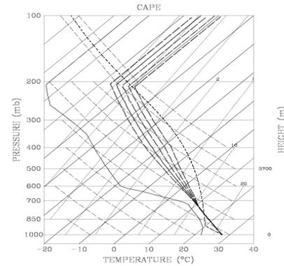
Fig.2: Soundings for five experiments. The long-dashed line from right to left are for CP1, 2,3, and 4, respectively. The solid line among the dashed lines is for the CNTL case.
