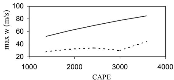
Fig. 4: The maximum vertical velocity (m/s) with respect to CAPE from the formula of ( $w = \sqrt{2CAPE}$ ; solid line;  $W = \sqrt{2CAPE}$ ) and from model simulations (dashed line).
