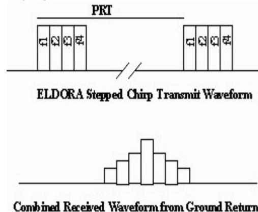
Figure 1. ELDORA transmit and received waveforms.
