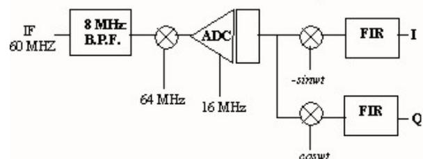
Figure 2: Block diagram DIGIF and Bandpass Filter.
