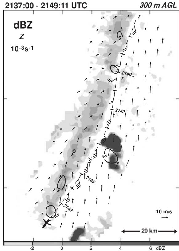
Fig. 7. Doppler wind synthesis for 2137:00 - 2149:11 UTC on June 19.
