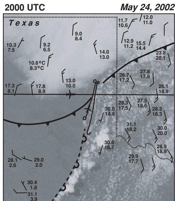
Fig. 1. Surface analysis at 2000 UTC 24 May 2002 superimposed onto a visual satellite image. The west-east and north-south lines represent the the DC-8 and P-3 flight tracks, respectively.
