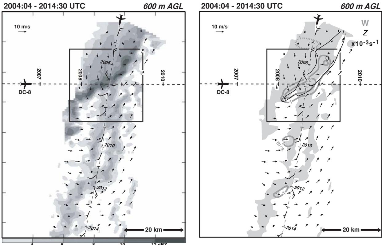
Fig. 3. Doppler wind synthesis for 2004:04 - 2014:30 UTC on May 24. The echoes stronger than 4 dBZ are shaded gray on the right. Vertical velocities and vorticity are shown on the right.
