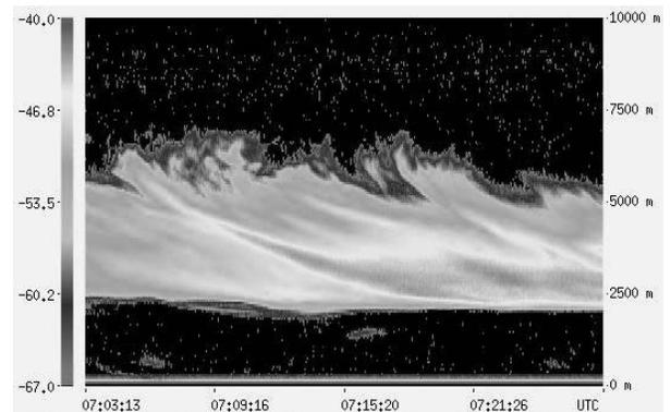
Figure 5. Time/height plot of backscattered power (uncalibrated reflectivity) for an ice cloud passing over Amherst, MA, December 25, 2002.
