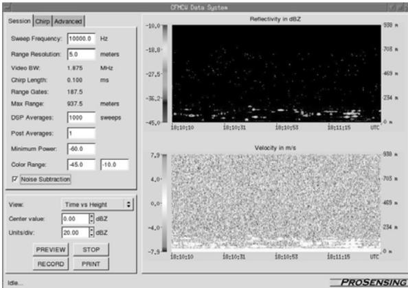
Figure 4. Graphical user interface for radar control and display of data products. Time/height plots of reflectivity and velocity for insects gathered April, 2002 in Amherst, MA are shown with the system configured for 5 m height resolution, 10 kHz PRF, and 0.1 s averages.
