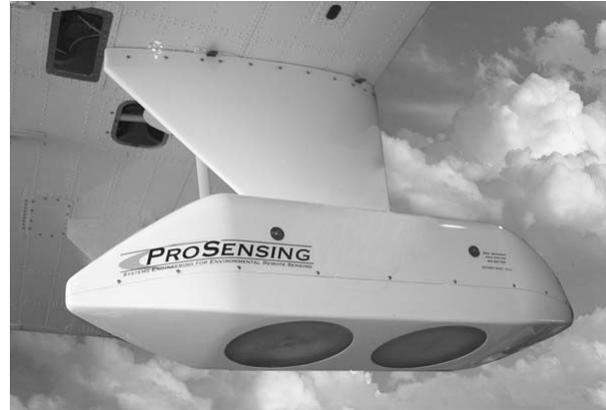
Figure 1. 95 GHz cloud radar mounted on the wing of the CIRPAS Twin Otter.
