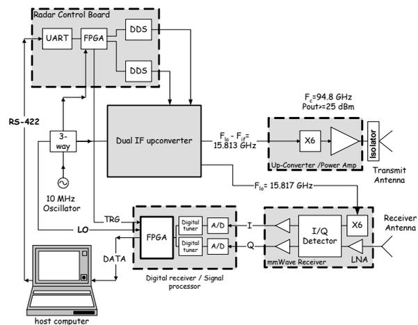
Figure 2. FMCW cloud radar system block diagram.
