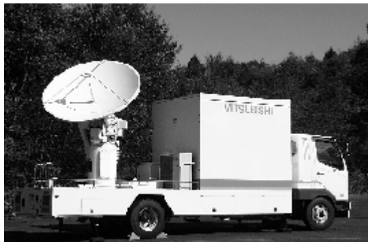
Fig. 1: Ka-band meteorological Doppler radar.
