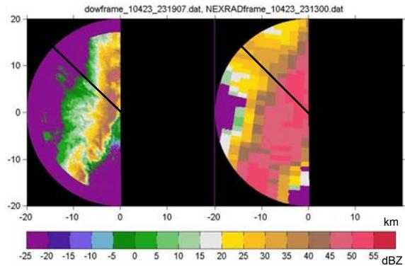
**Figure 5.** Horizontal cross-section of storm reflectivity as seen by the DOW at 2319 UTC (left) and the KNQA at 2313 UTC (right) radar on 23 April 2001.
