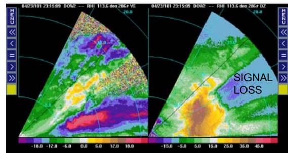
**Figure 6.** Vertical cross-section of radar radial Doppler velocity (left panel) and reflectivity (right panel) as observed by the DOW radar on 23 April 2001 at 2315 UTC. The resolution is 50 m in the radial direction and 1 deg in azimuth. Range rings are shown at 5 km intervals.
