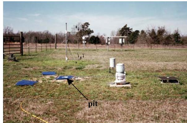
**Figure 2.** Climatological station (station 50) in the catchment center includes above-ground and buried rain gauges, a disdrometer, wind profile measurements, and a SURFRAD station.
