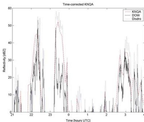
**Figure 7.** Reflectivity based on disdrometer observations at station 50 and closest pixel of DOW and KNQA radar.
