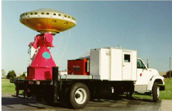
**Figure 3.** Doppler-on-Wheels (DOW) radar of the University of Oklahoma (deployment site marked by rectangle at upper end of catchment in Fig. 1).
