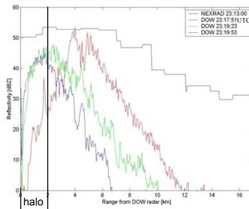
**Figure 8.** Reflectivity vs. distance from the DOW for both the time corrected KNQA and DOW radar.
