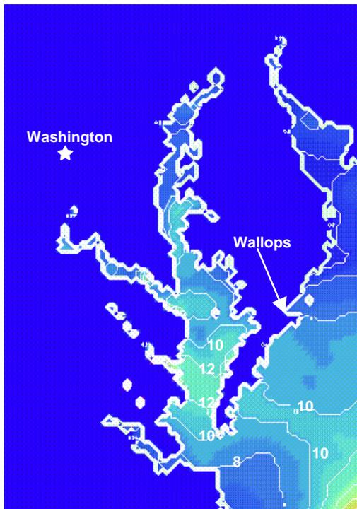
Fig. 5 Evaporation Duct Height (EDH) (m) on the 3 km COAMPS grid at 00 UTC 11 Apr 2000.
