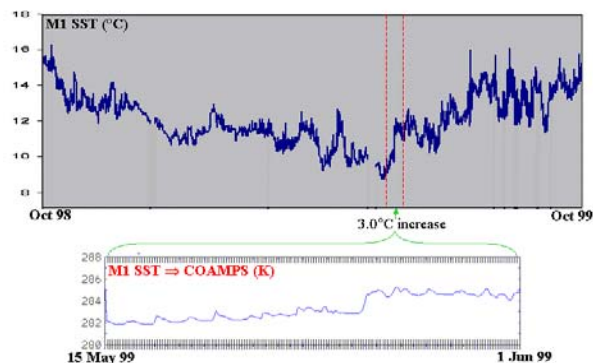
Figure 1: M1 buoy measurements of SST ( ^{\circ}\text{C} ) for Oct 98 - Oct 99, and COAMPS™ SST (K) 15 May - 1 Jun 99.
