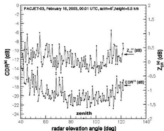
Figure 5. Differential reflectivity ( $Z_{DR}$ ) and circular depolarization ratio (CDR) estimate for an RHI scan by the X-band radar through a deep BB-producing cloud.
