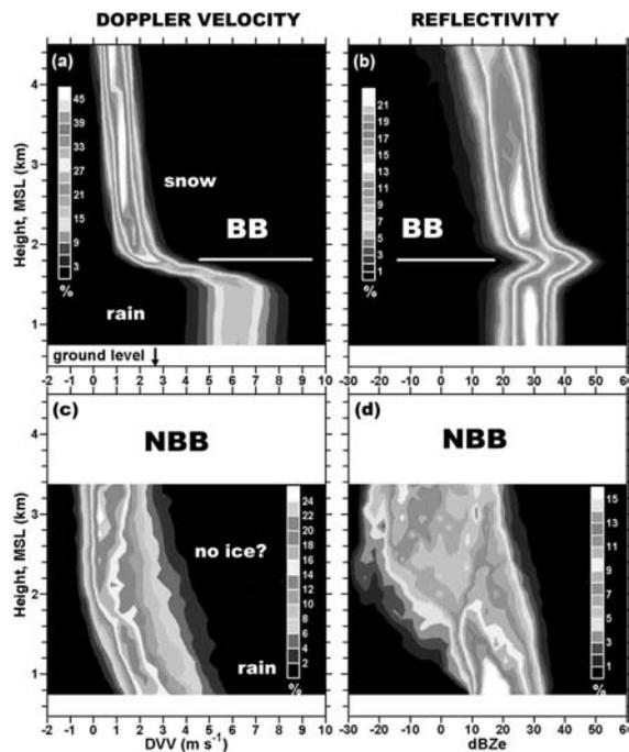
Figure 1. Height-normalized composite of S-band profiles of reflectivity and vertical Doppler velocity from the entire CALJET winter season showing distinct differences in bright band (top) and non-bright band (bottom) cases. The average rain rate was  $4 \text{ mm hr}^{-1}$  for each composite. After White et al. (2003).
