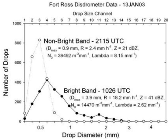
Figure 3. Drop size spectra from the disdrometer for two 1-minute periods during bright-band and non-bright-band periods of rainfall.
