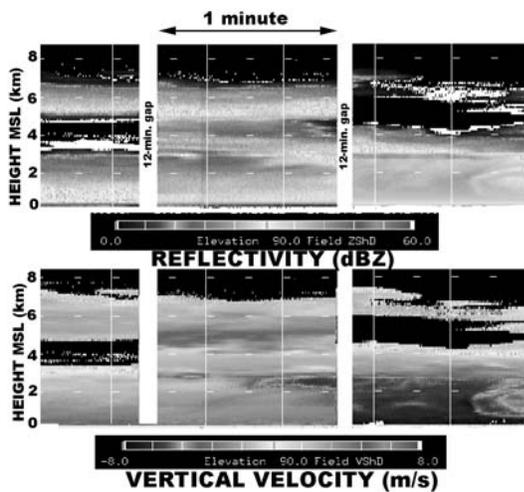
Figure 4. Three short periods of vertical data from the X-band radar on 13JAN03 between 1002 and 1029 UTC showing rapid development of the bright band as a higher cloud moved over the persistent lower stratus at Fort Ross. Time proceeds from left to right in each panel.
