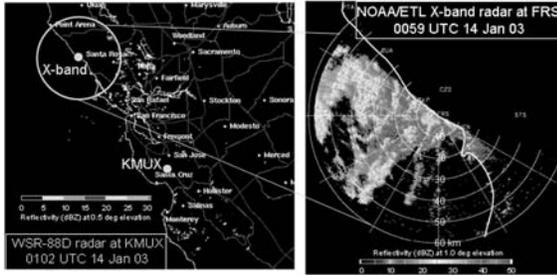
Figure 6. Comparisons of scan images from the San Francisco NEXRAD (left) and the PACJET X-band radar (right) at Fort Ross showing the shallow precipitation echoes that passed beneath the NEXRAD coverage.
