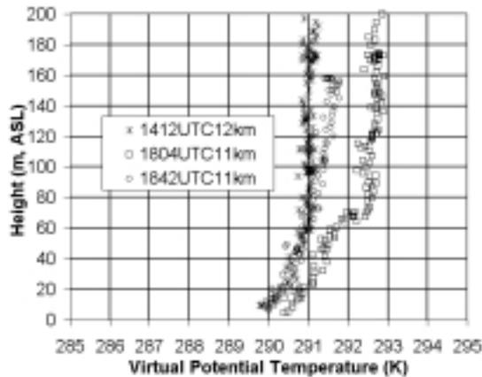
**Figure 11: Profiles of Virtual Potential Temperature near 11 km offshore at 1412 UTC, 1804 UTC and 1842 UTC.**
