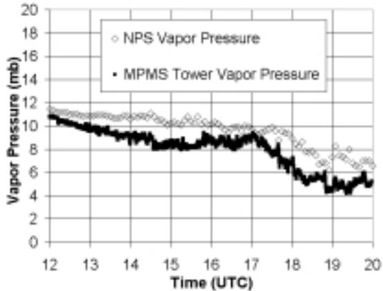
**Figure 7: Water vapor pressure measured on the beach and 13 km offshore on April 30.**
