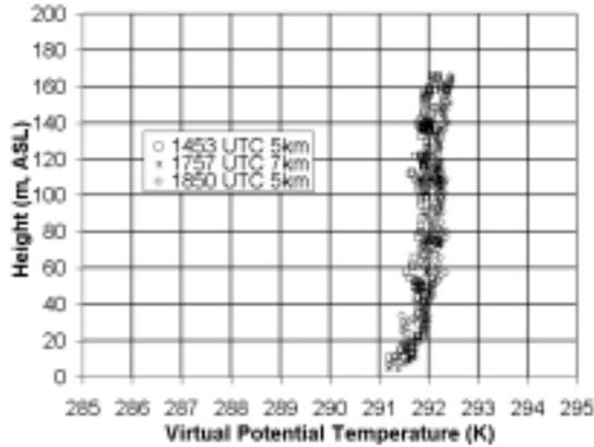
**Figure 10: Profiles of Virtual Potential Temperature near 6 km offshore at 1453 UTC, 1757 UTC and 1850 UTC.**
