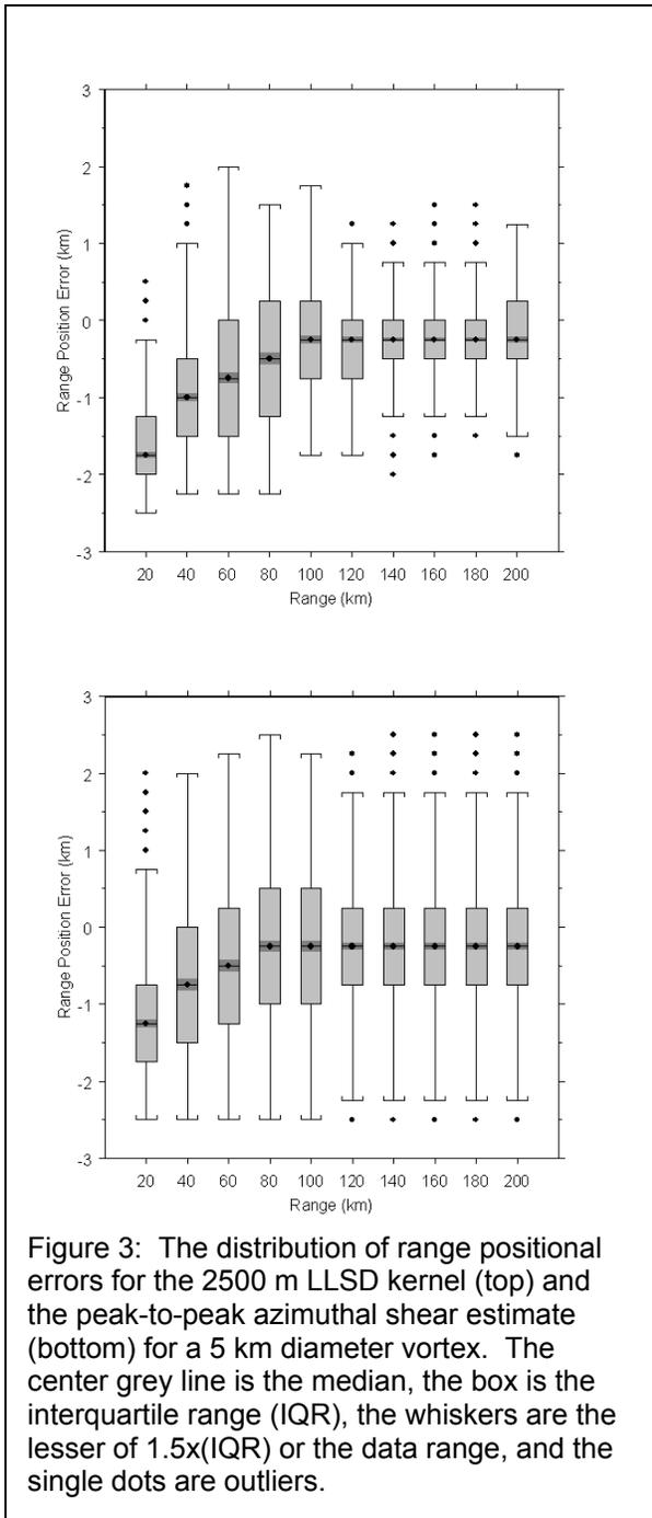
Figure 3: The distribution of range positional errors for the 2500 m LLSD kernel (top) and the peak-to-peak azimuthal shear estimate (bottom) for a 5 km diameter vortex. The center grey line is the median, the box is the interquartile range (IQR), the whiskers are the lesser of 1.5x(IQR) or the data range, and the single dots are outliers.
