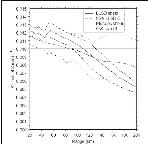
Figure 1: Mean and 95% confidence limits for LLSD and peak-to-peak estimates of azimuthal shear at the vortex center for a 5 km diameter vortex with half vorticity of  $0.01 \text{ s}^{-1}$ .
