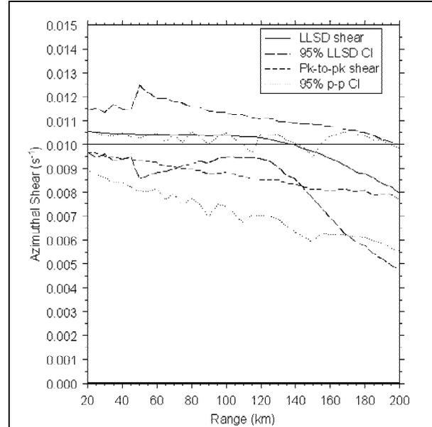
Figure 2: Mean and 95% confidence limits for LLSD and peak-to-peak estimates of azimuthal shear at the vortex center for a 8 km diameter vortex with half vorticity of  $0.01 \text{ s}^{-1}$ .
