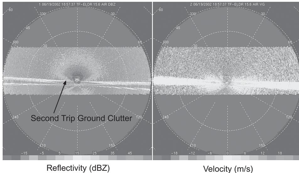
**Figure 1.** Eldora data from IHOP on 19 June 2002 showing second trip clutter echo contamination. Aircraft altitude is about 3 km AGL and range rings are 15 km.
