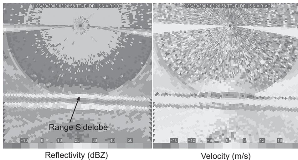
**Figure 2.** Eldora data from IHOP on 20 June 2002 showing range sidelobe contamination near the surface. Aircraft altitude is 3 km AGL.
