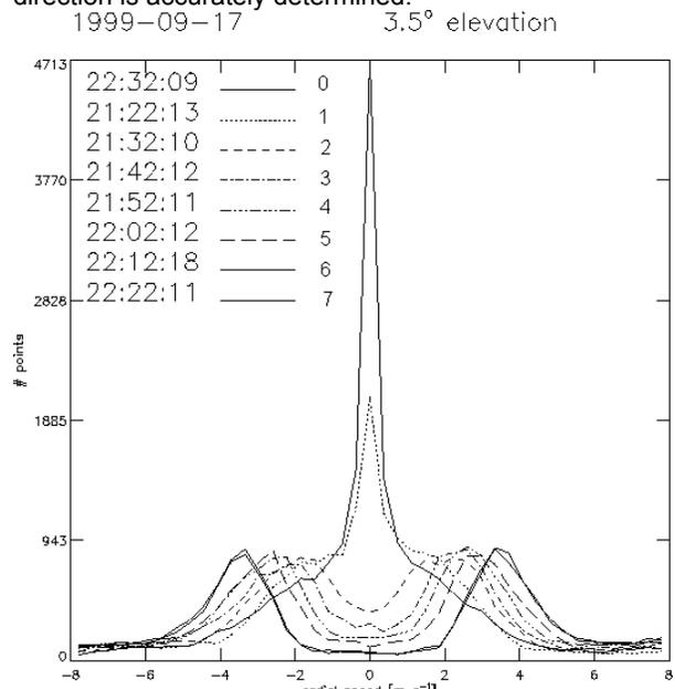
Figure 2: Radial velocity histogram for different clutter filters during a clear air echo case.
