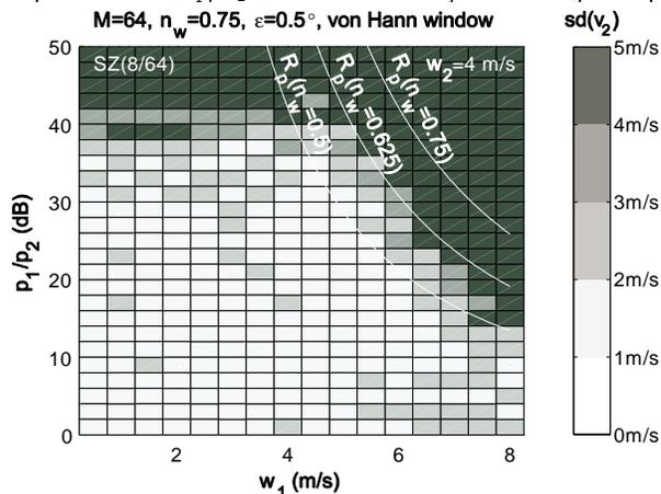
Figure 2: The standard deviation of the recovered velocity  $\hat{V}_2$  as a function of the power ratio  $P_1/P_2$  and the width of the stronger trip signal,  $W_1$ . Reproduced from Sachidananda and Zrnić (1999).
