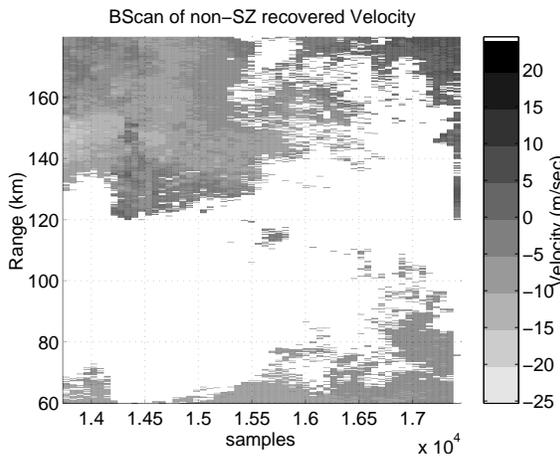
Figure 6: Concatenated B-scans of velocity as would be measured by the current WSR-88D scanning parameters. The velocity is calculated from the truth fields of Figs. 3 and 4 (top panels) and can be compared to the SZ(8/64) recovered velocity of Fig. 4, bottom panel. The large white area is censored data.
