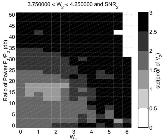
Figure 1: The standard deviation of the errors of the recovered weak trip velocity ( $\hat{V}_2$ ) as a function of the power ratio  $P_1/P_2$  and the width of the stronger trip
