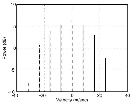
Figure 8: Spectrum of the modulation code after 3/4 notch filter and recohering. Solid lines are without clutter filtering the dash lines are with clutter filtering.
