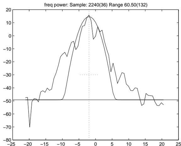
Figure 3: Experimental weather spectrum with estimated Gaussian curve overlaid.
