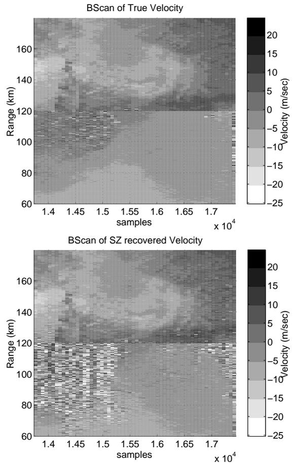
Figure 5: Concatenated B-scans of the radial velocity. The seam between the 2 separate scans can be seen at the 120 km range gate. Top Panel: Truth velocity; Bottom Panel: SZ(8/64) recovered velocity.
