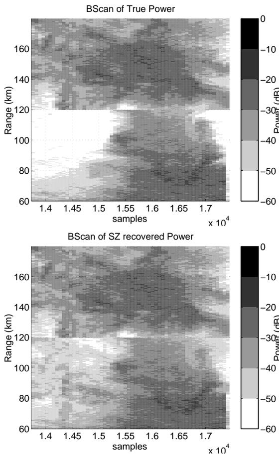
Figure 4: Concatenated B-scans of power. The seam between the 2 separate scans can be seen at the 120 km range gate. Top Panel: Truth raw  $I^2 + Q^2$  power. Bottom Panel: SZ(8/64) recovered power.
