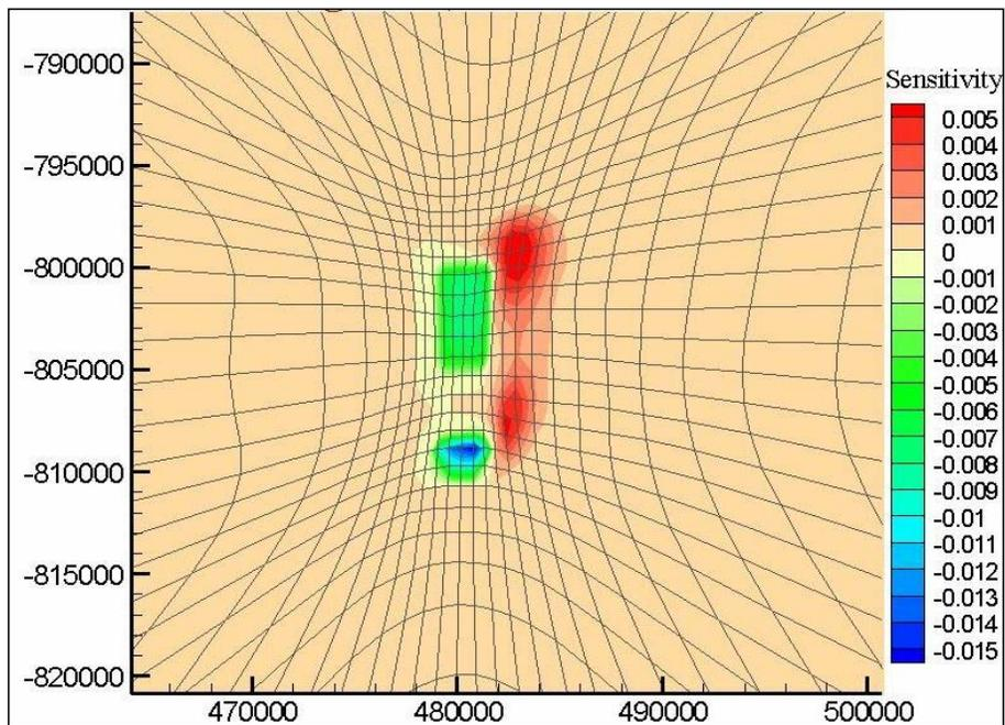
**Figure 5** Adaptive Grid Result for Direct Sensitivity of O<sub>3</sub> (ppm) to Fire Emissions
