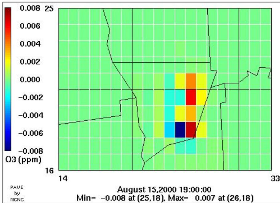
**Figure 4** Static Grid Result for Brute Force Sensitivity of O<sub>3</sub> (ppm) to Fire Emissions
