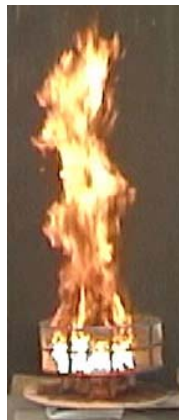
Fig. 3. Fire plume of live chamise shrub fuel. The experimental set up including fuel container, thermal insulation barrier and digital weight scale is illustrated.
