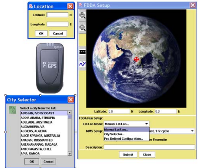
FIG. 2. The graphical interface that is used for setting up the geographic area coverage for model forecasts. The user can manually enter a latitude and longitude, or by using GIS-based tools to select the area of interest. The version of the system that runs on a PDA incorporates a portable GPS receiver that can be used to acquire the geographic coordinates.
