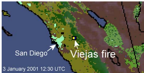
Figure 2: GOES-10 WF_ABBA image of the Viejas fire (3 January 2001) at the time it was first detected, 12:30 UTC. The fire start time was reported to be 12:24 UTC.
