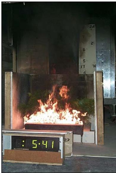
Figure 2. Intermediate scale biomass calorimeter at University of California Forest Products Laboratory used to measure combustion characteristics of small shrubs using oxygen consumption calorimetry.
