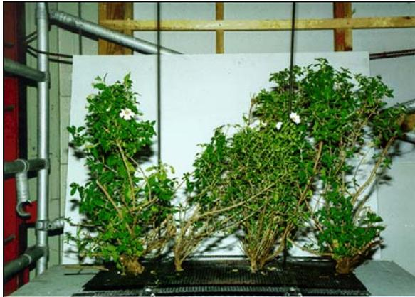
Figure 6. Arrangement of plants used in Intermediate Scale Biomass Calorimeter tests.
