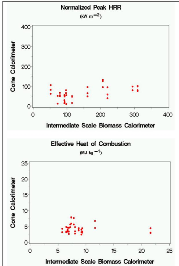
Figure 7. Relationship between PHRR and AHOC measured by a Cone Calorimeter and an Intermediate Scale Biomass Calorimeter.
