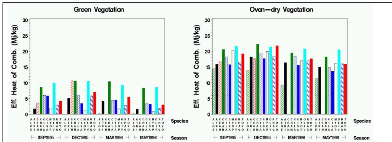
Figure 5. Mean effective heat of combustion (HOC) for green and over-dry samples of ornamental vegetation in southern California. HOC determined using 25 kW m<sup>-2</sup> flux in a cone calorimeter.
