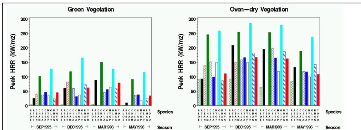
Figure 4. Mean peak heat release rates (HRR) for green and oven-dry samples of ornamental vegetation in southern California. Peak HRR determined using  $25 \text{ kW m}^{-2}$  flux in a cone calorimeter.
