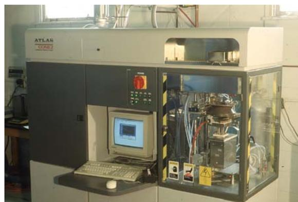
Figure 1. Cone calorimeter located at USDA Forest Service Forest Products Laboratory used to measure combustion characteristics of various vegetation specimens.
