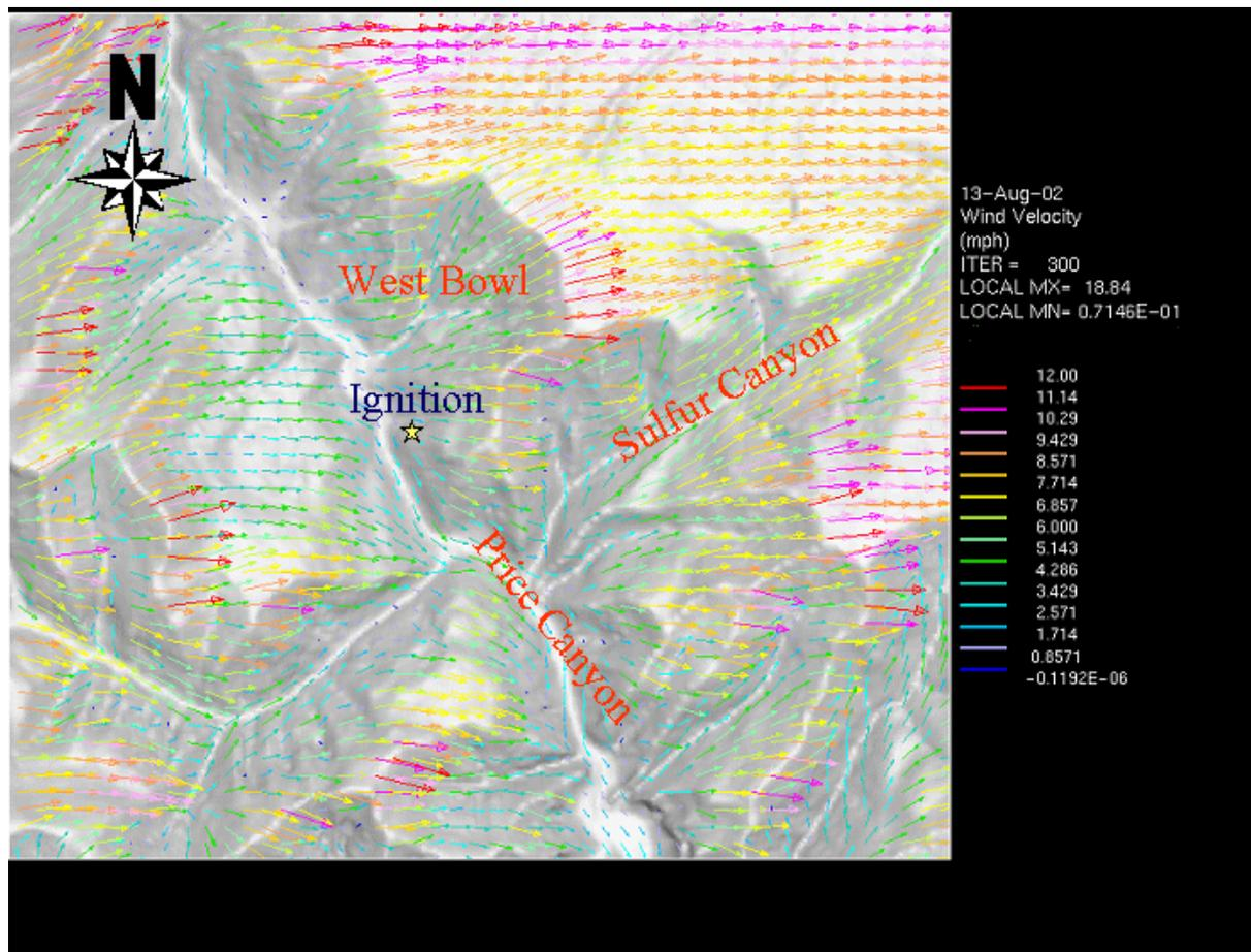
Figure 1--CFD simulation of 50-meter height wind velocities of the Price Canyon Fire area.
