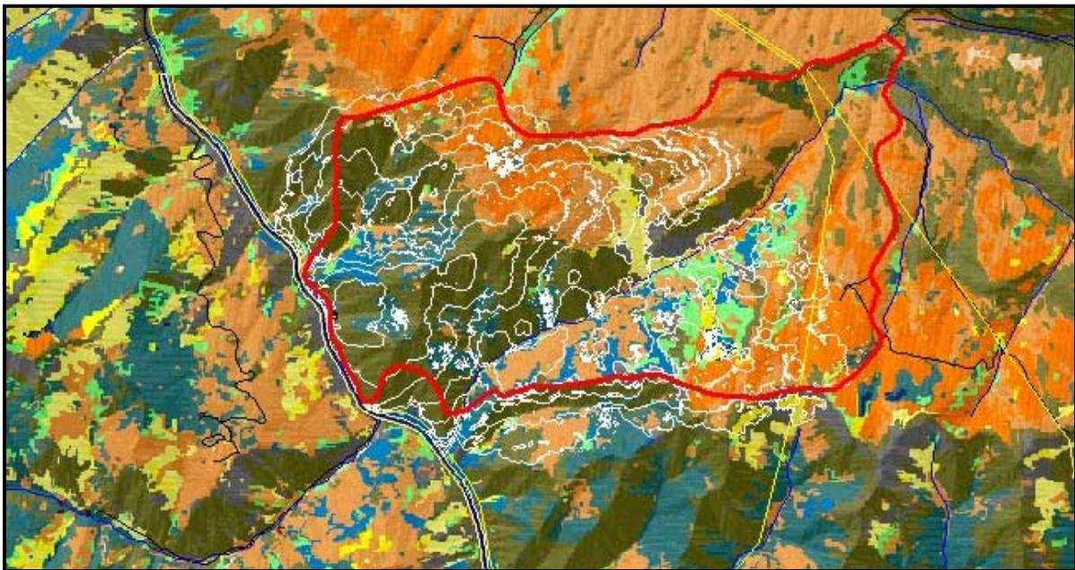
Figure 3--FARSITE simulation of the 2022 Price Canyon Fire using gridded winds produced by commercial CFD software.
