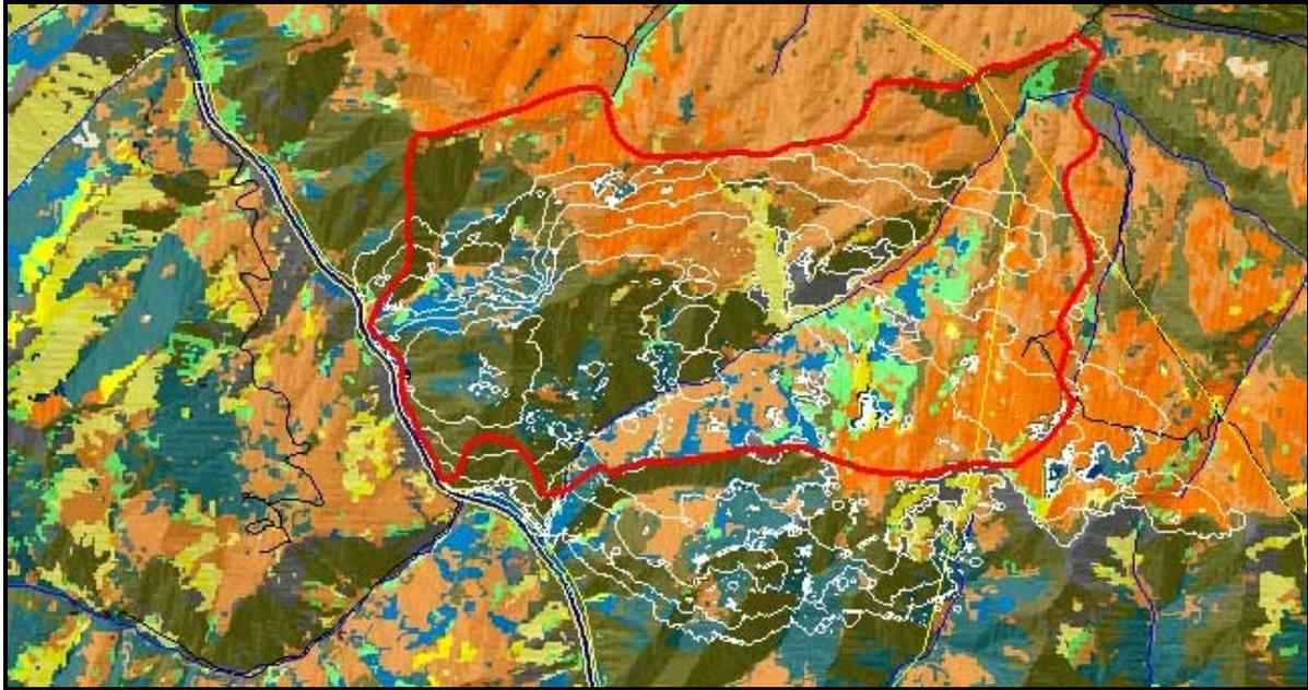
Figure 2--FARSITE simulation of the 2022 Price Canyon Fire using constant speed and direction winds.
