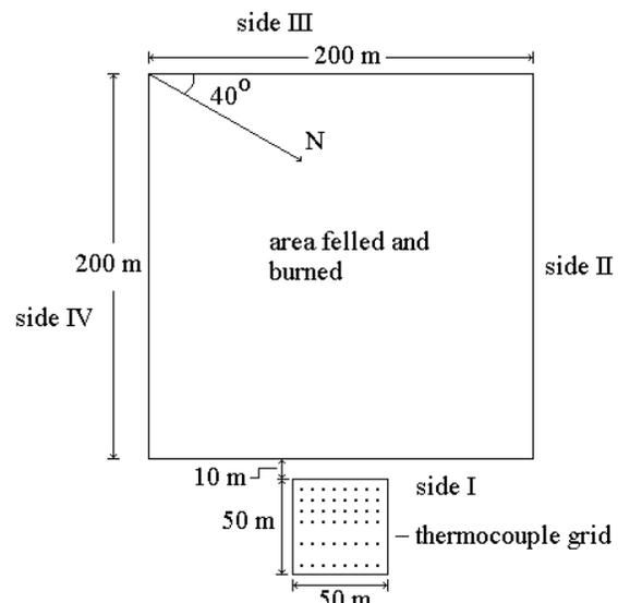
Figure 2 - Test plot F and the location of the thermocouple grid.
