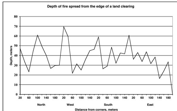
Figure 5. Depth of understory fire spread from the edge of a primary forest with an ignition source from an experimental slash burn in Alta Floresta, Brazil in 2001. The slash burning unit was a 200 x 200 m plot.
