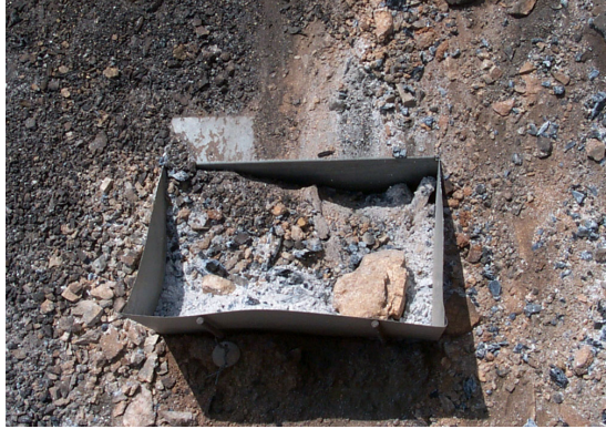
Figure 2. Post-fire dry season erosion captured in a 30-cm aperture sediment collector.
