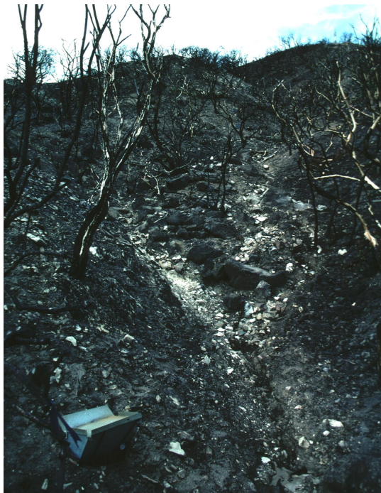
Figure 3. Post-fire wet season erosion in a burned chaparral watershed. Note collector trap with cover for scale and scour from overland flow.
