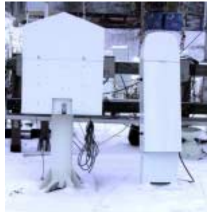
Fig.3. Outdoor test setup with a CT12K and the new ceilometer in December 2002.
