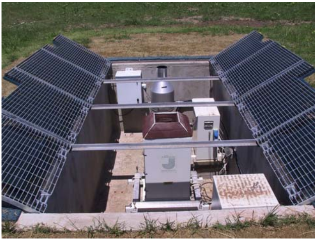
Fig. 3 The inside of the pit showing the disdrometer (front) and Geonor gauge (back).
