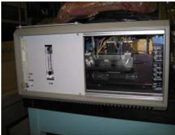
Figure 4. Control module showing internal reference (lower) and calibration (upper) cells.
