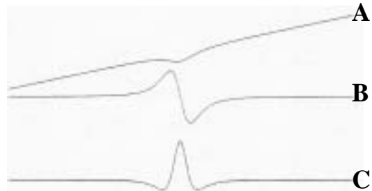
Figure 5. Normal absorption feature (A); first harmonic, 1f (B); and second harmonic, 2f (C).
