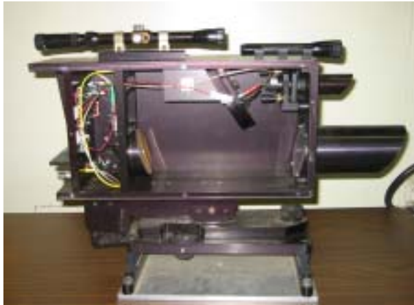
Figure 2. Telescope assembly used to launch the diode laser beam.
