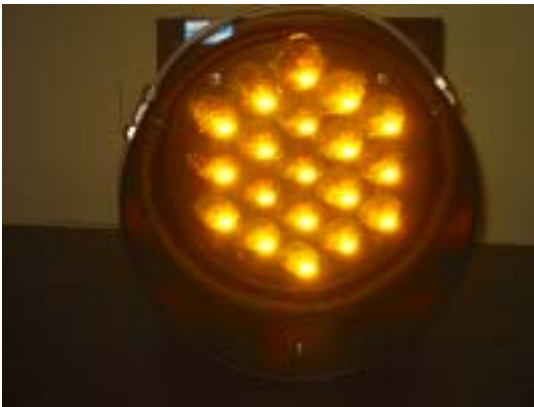
Figure 3. Retro-reflector assembly used to return the divergent diode laser beam to the telescope.
