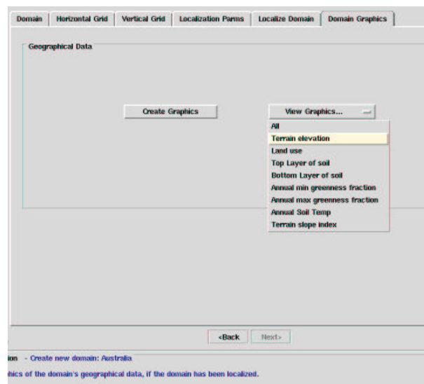
Figure 11. Display of Domain Graphics panel. This user has NCAR Graphics NCL available and is able to create and view output from domain localization.
