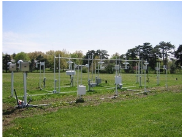
Fig. 1. Instrumentation illustration: the array of air temperature monitoring systems used (USCRN PRT sensors and shields, two RMY systems, one PMT system, two ASOS 1088 as well as two MMTS systems) at the experimental field.
