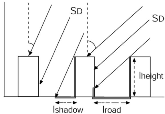
Fig. 3: Radiation in the urban street canyon.  $I_{shadow}$  and  $I_{road}$  are the length of shading on the road, respectively.  $I_{height}$  is the building height.
