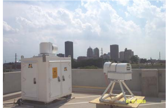
Figure 3. Photograph of the ARL Microwave Radiometer (right) and the ARL Wind Tracer Lidar (left) measuring radial wind velocities over the Central Business District of Oklahoma City. (Photograph by Young Yee).
