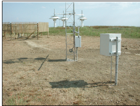
Figure 2. Aspirated Shields each containing one PRT
