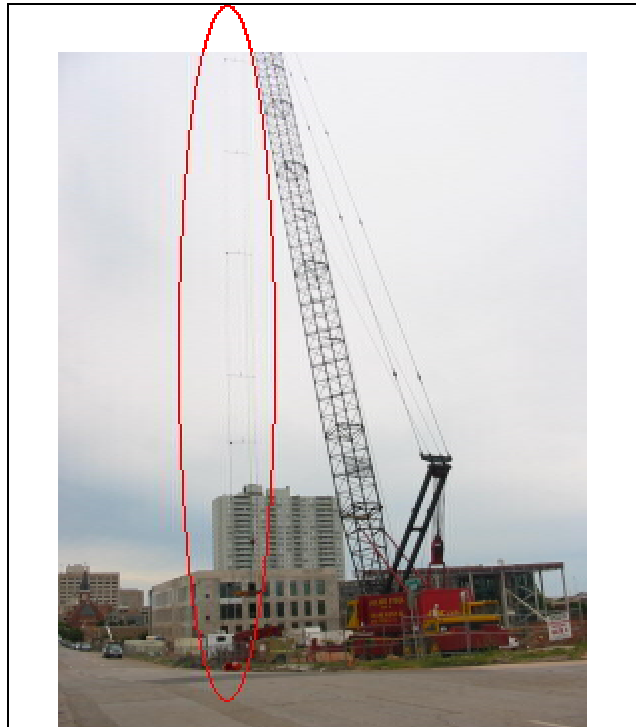
Figure 1: The pseudo-tower, outlined in red, supported by a crane to the north of the pseudo-tower. The view is to the south-west. Most winds during the JU2003 experiment were from the south. (Photo courtesy of M. Leach, LLNL.)
