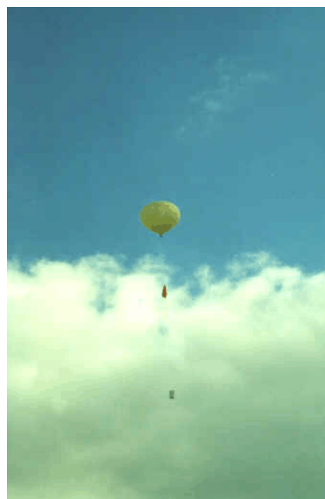
Figure 1 a-d. Photos of radiosondes. Top left, radiosonde being prepared for release. Top right, radiosonde being released. Bottom left, radiosonde flight underway with, in foreground, the balloon inflation shelter with radome above it that houses the radiosonde tracking equipment. Bottom right, radiosonde in full flight. By the time the balloon bursts two hours and approximately 35 vertical kilometers later the balloon will be 6 meters in diameter. Photos courtesy of the Upper-air Observations Program, Observing Systems Branch (OSB), NWS.
