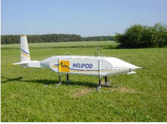
Fig. 2: The helicopter-borne turbulence measurement system Helipod is an autonomously operating sensor system, attached to a 15 m rope. It operates at 40 \text{ ms}^{-1} air speed and measures wind vector, temperature, and humidity at a rate of 100 Hz.
