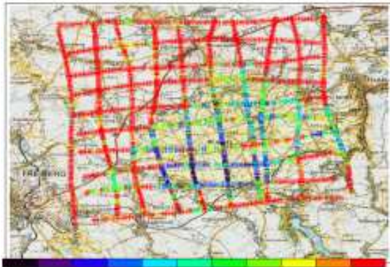
Fig. 8: Grid flight pattern during the Tharandt experiment. This pattern was flown when the convective BL was already established. The difference of wood and grass land is clearly visible by surface temperature (colors) measured by the Do 128 aircraft.
