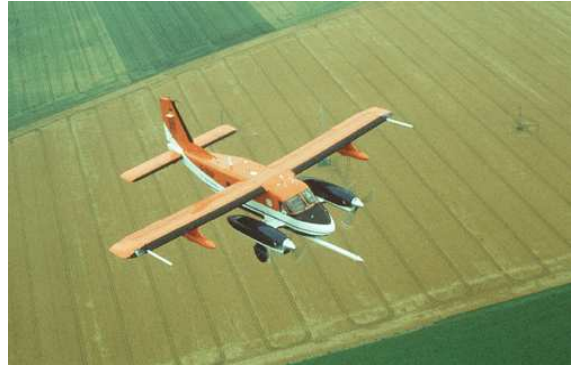
Fig. 3: The research aircraft Do 128 recently received new equipment. The aircraft operates at an air speed of 60 m/s and samples data at 100 Hz.
