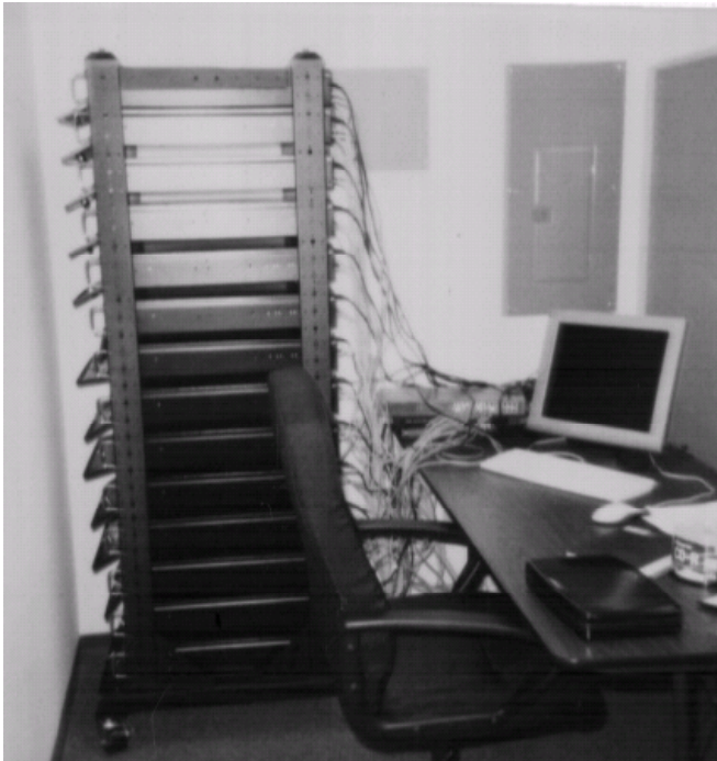
Figure 1. A fourteen-node Beowulf parallel computing cluster, Charlotte , at RESPR.
